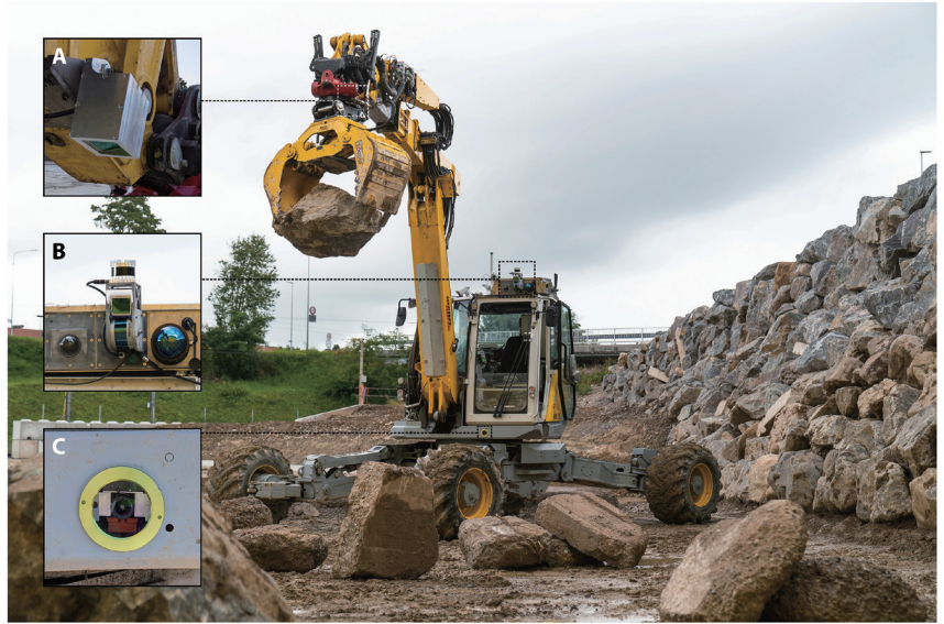
A: Arm-mounted Livox Mid-70 sensor, B: rooftop perception box with multiple LiDAR sensors and camera, C: lower-cabin camera
